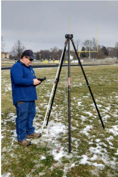
*Illustration 2: HIC Testing of a Natural Turf Field During*
