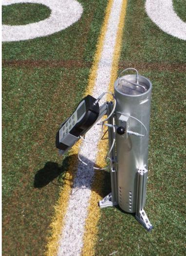
*Illustration 1: G-max test equipment on an infilled system with coconut fiber.*
