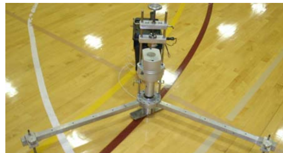
Illustration 1: Shock Absorption and Thickness Test Equipment
