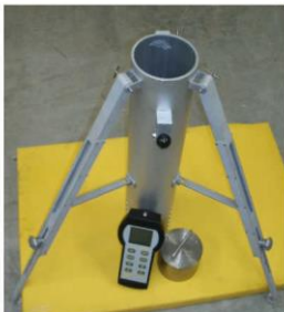
Impact Test Equipment for Athletic, Gymnastic and Trampoline Mats, Pads, and Pits
