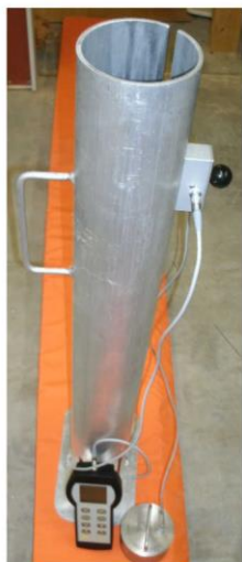
Impact Test Equipment for Athletic, Gymnastic and Trampoline Mats, Pads, and Pits
