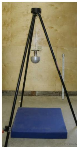
Impact Test Equipment for Athletic, Gymnastic and Trampoline Mats, Pads, and Pits
