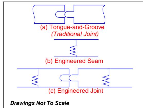
Figure 1: Joint Schematics
