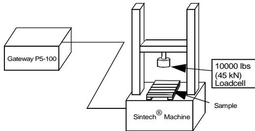
**Figure 2: Schematic of materials test setup.**
