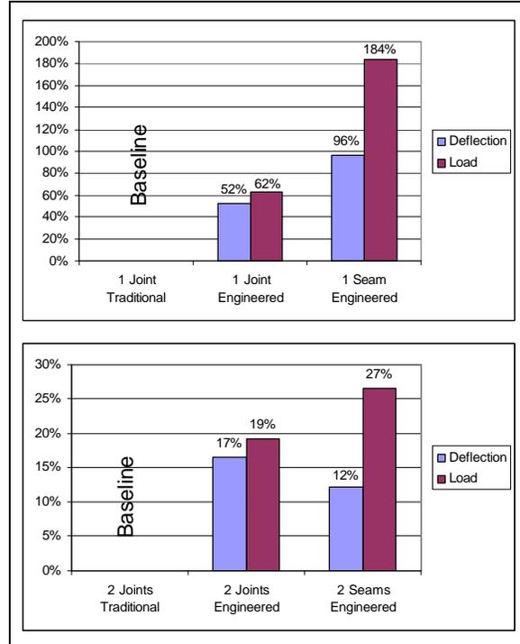
**Figure 6: Percent Increases Provided By 25/32" Engineered Strip Flooring Over 25/32" Traditional Strip Flooring.**
