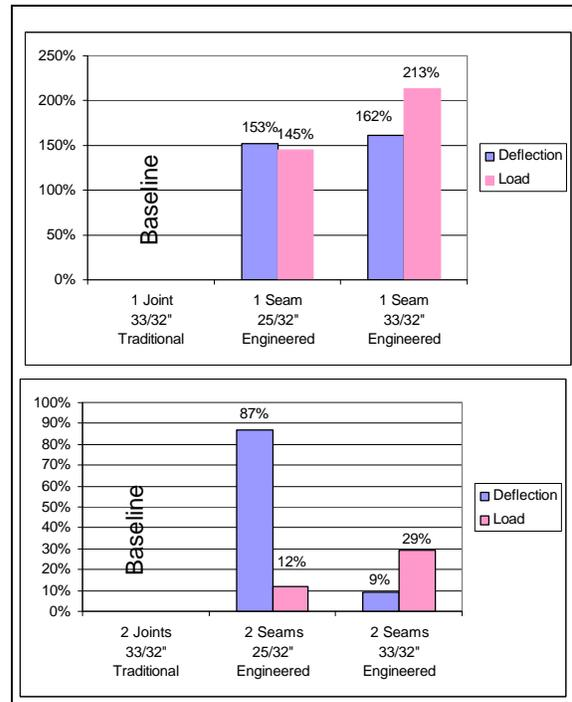
Figure 7: Percent Increases Provided By Engineered Seams in 25/32" and 33/32" Engineered flooring strips over 33/32" traditional joints.
