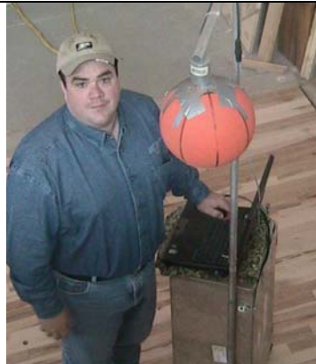
Founder Paul Elliott, Ph.D., P.E. with a ball rebound test device.
